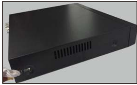
① Loosen the screws to open the cover.
