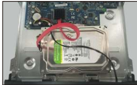
④ Connect the power and data cables.
