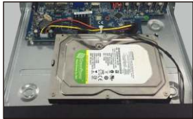
③ Put the HDD onto the bottom of the device.
