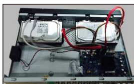
④ Connect the power and data cables.
