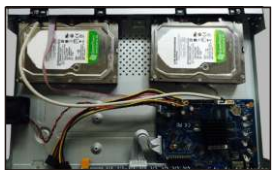
③ Place the HDDs onto the bottom of the case.
