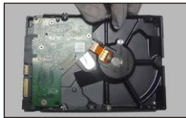
② Screw the screws into the holes of HDD but not tighten them.
