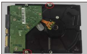
② Screw two screws into the holes of HDD but not tighten them.
