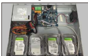
④ Install the other three HDDs according to above-mentioned method.
