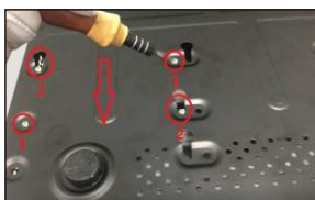
③ Turn over the machine and place the HDD with two screws onto the bottom of the case. Then lock the screws according to the order of the marks.
