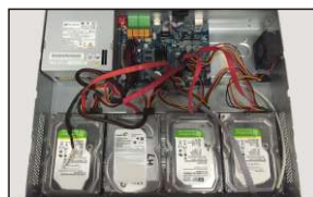
⑤ Connect the power and data cables.
